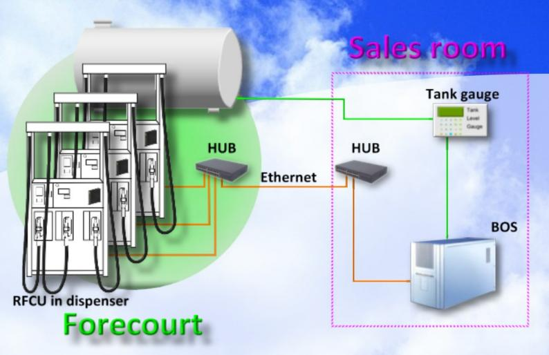
After RFCU be installed into dispensers in fore-court, all dispensers' communication interfaces become to Ethernet, connect these dispensers to a switch HUB then only need 1 LAN cable connect to back office. Due to LAN cable is very popular and standard, very easy to get and replace.
