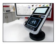
The ACR123U is the USB version of the cost-effective, flexible and intelligent contactless reader ACR123S. It can be integrated to existing (Point-of-Sale) terminals or cash registers to offer the convenience of a cashless payment system. Developed based on the 13.56 MHz contactless (RFID) technology, it supports any contactless card following the ISO 14443-4 standard.
