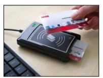
ACR1281U-C1 DualBoost II is the second generation of ACS's ACR128 DualBoost Reader. It is a dual interface reader that can access any contact and contactless smart cards following the ISO 7816 and ISO 14443 standards. ACR1281U-C1 enables one to conventionally integrate separate and independent applications for contact and contactless technologies into one device and one card.
