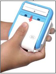
Remove the cover completely to reveal all three available SAM slots.
